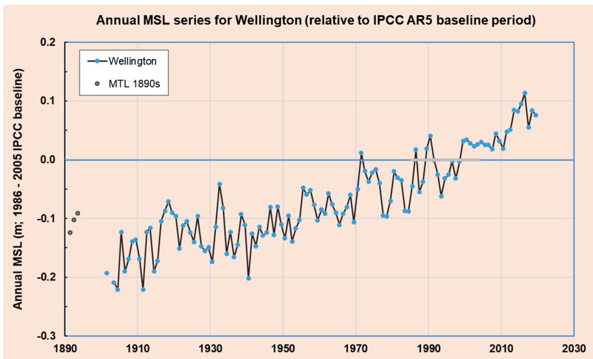
**Figure 2-1: Annual MSL series from 1891 to 2019 for Wellington Harbour.** *Source:* Original measurements: GWRC and LINZ; Processed annual MSL: Hannah and Bell (2020), J. Hannah (pers. com. for 2019 value). *Note:* values for 1891–1893 are sourced from archives listing only monthly averages of low and high tides (MTL), which are less reliable as a measure of MSL than more frequent data (Hannah 2004).
