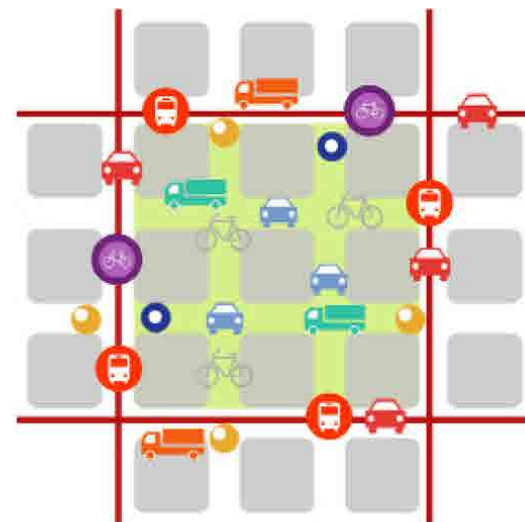
Barcelona example: Although Wellington does not have a the same extent regular block pattern, the principles of neighbourhoods that are internally programmed for slow local movement and an arterial for wider network movements is part of the Vision
