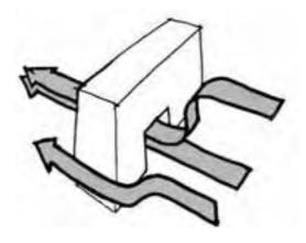
The zone of discomfort is not confined to the passages themselves but could extend over approximately the same area as that of the opening on the lee side, the air being released in the form of a localised jet. These "slots" under buildings make for more directional airflows than when the building has guide walls or is on columns.
