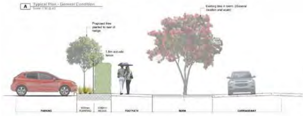
B Typical Section - General Condition Scale: 1:50 @ A3
