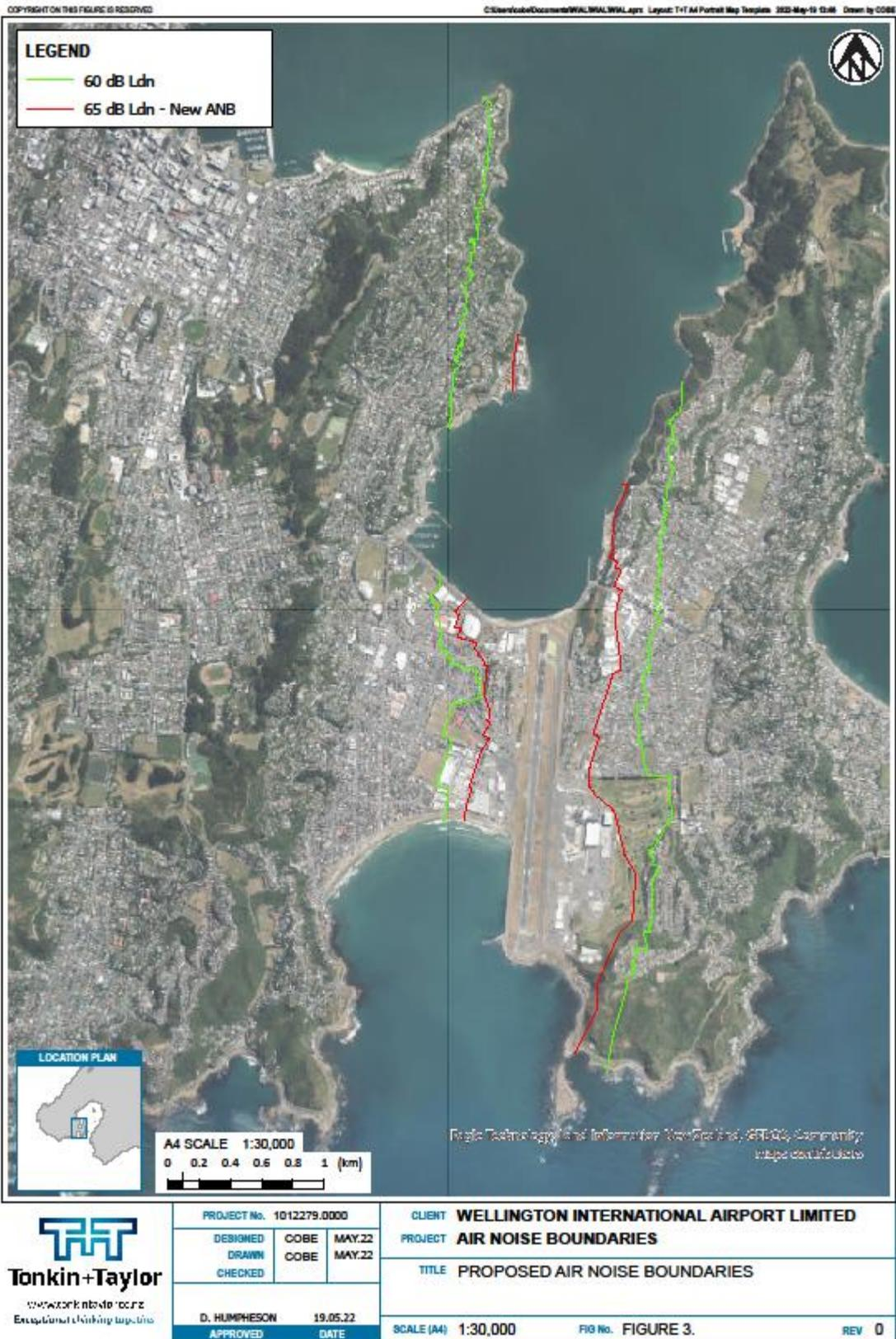
**Figure 1** T&T predicted 2050 aircraft noise contours for WIA – showing 60 dBA Ldn and 65 dBA Ldn contours.
