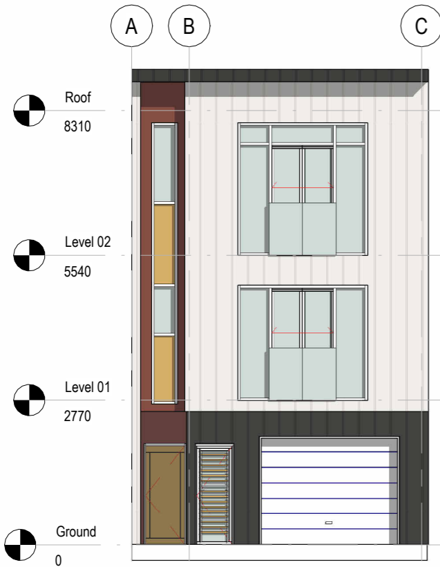
04 Front Elevation SCALE = 1 : 100
