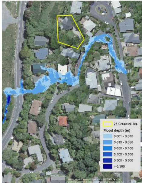
Figure 3: Updated flood modelling based on accurate topographic information including built features.
