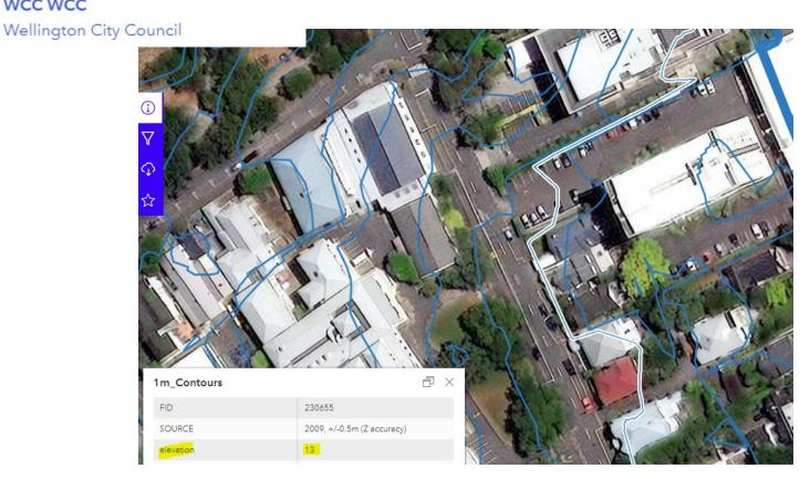
Where Tiakiwai has been incorrectly plotted in the PDP it is crossing Hobson St on a contour that is ~3m above the lowest point along this segment of the street.
