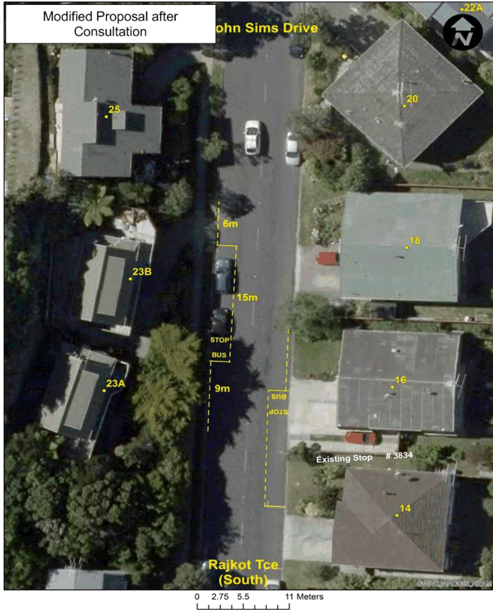
Bus Stop - At All Times John Sims Drive, BROADMEADOWS User Name: agatec Reference Scale: 1:300 Date: 29/08/2016
