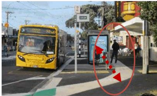
Figure 2-11: Photo showing a pedestrian waiting on the cycleway bus stop bypass
