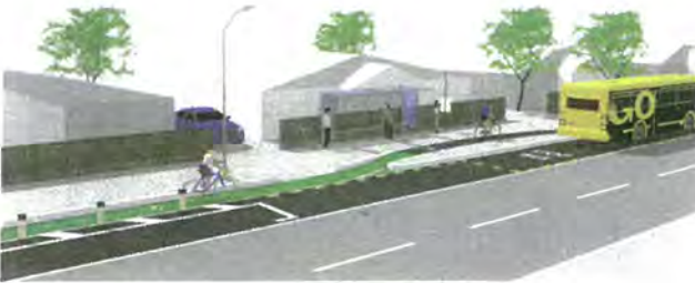
Bus stop bypass with dedicated cycle path.
