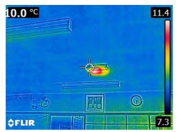
Infrared image of ceiling of main hall. Hot spot noted from ceiling mounted emergency lighting. (Not operational).
