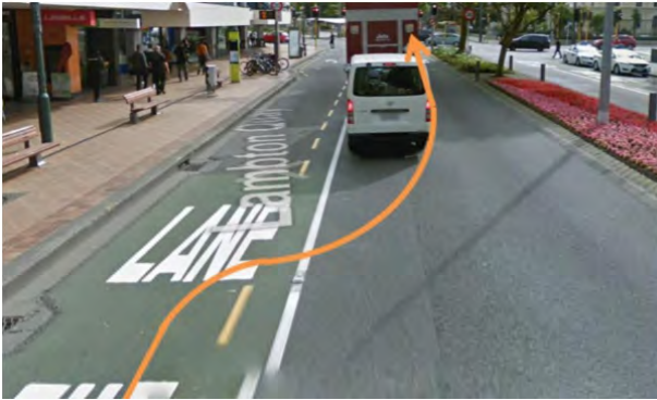
Figure 19: Weaving on the Northbound Approach to the Bowen Street Intersection
