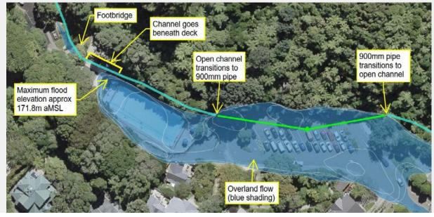
This modelling also gives guidance on the minimum cross sectional area required to accommodate the modelled stream flows in this rain event. A cross sectional area of 20m2 is required, in contrast to the 1.82 m2 currently provided. This provision is in addition to the building platform elevation. Further modelling of stream flow and downstream capacity may allow a lower building platform if flow paths can be improved.
