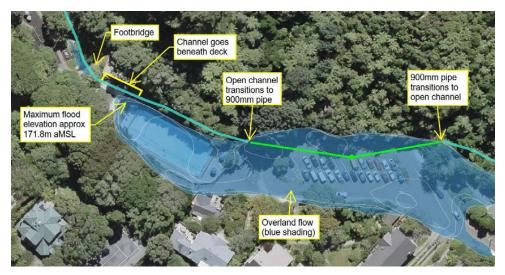
Figure 3.6 Flood Hazard Modelling completed by Wellington Water for the 1% AEP rain event + 20% rainfall depth for climate change, sourced from publicly available flood hazard mapping. Graphic marked up by T+T.
