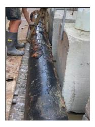
WW CI Rising Main – photo of failed piped showing longitudinal split - Victoria St July 2021
