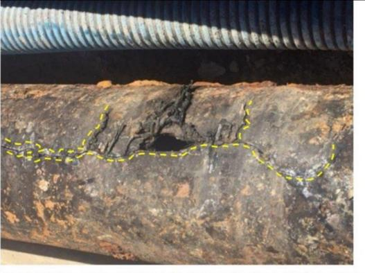
Figure 4b. Failed pipe sample shortly after recovery showing blowout and cracking. The yellow marks indicate the approximate position of the main cracks.
