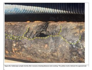
WW CI Rising Main – sample from pipe failure Victoria St November 2017
