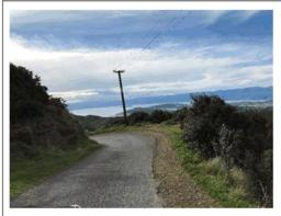
Photograph 3-11: Sharp corner with limited sight distance showing edge break and overrun
