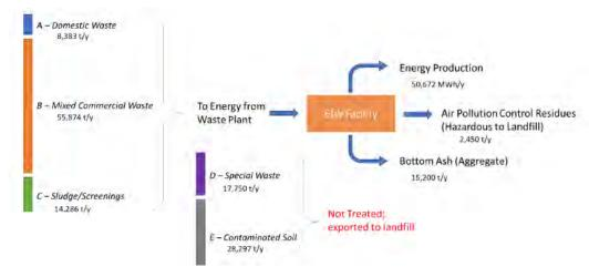
HOW WASTE TO ENERGY INCINERATION WORKS
