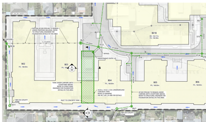
Figure 25: Location of detention tank (green hatching).
