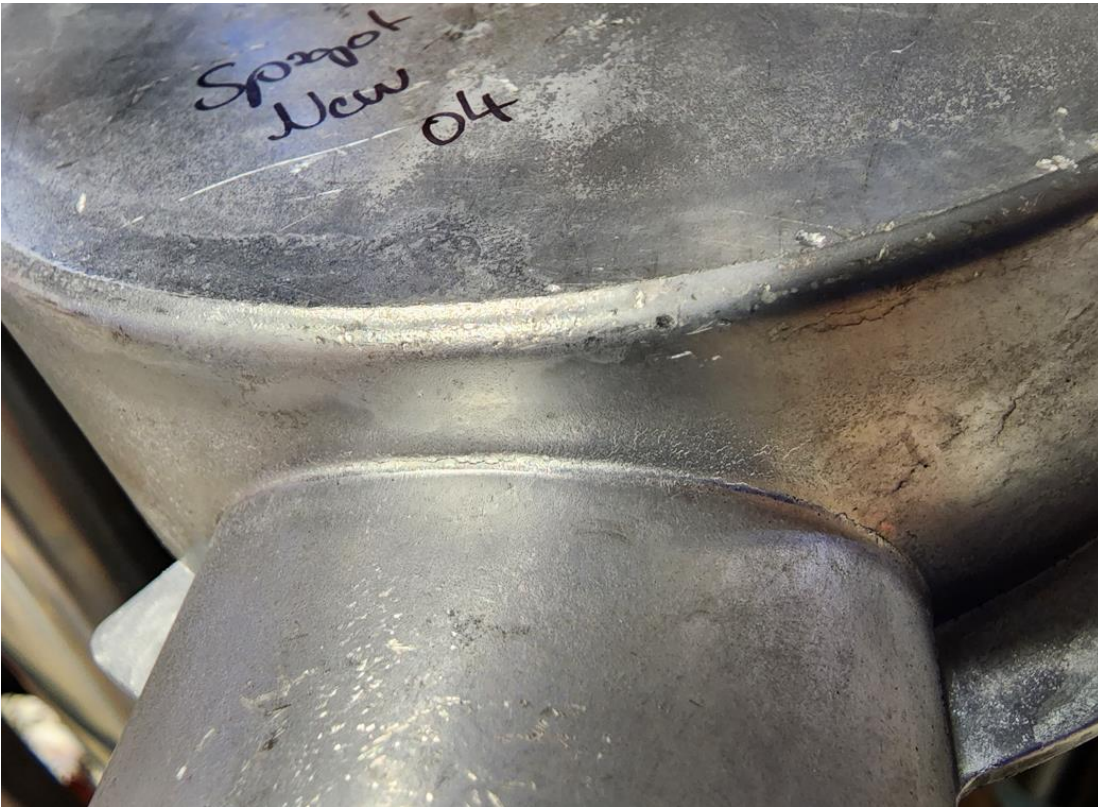
Figure 18 - Fourth sample with cracking
