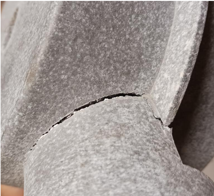
Figure 7 - Vertical Load Failure
