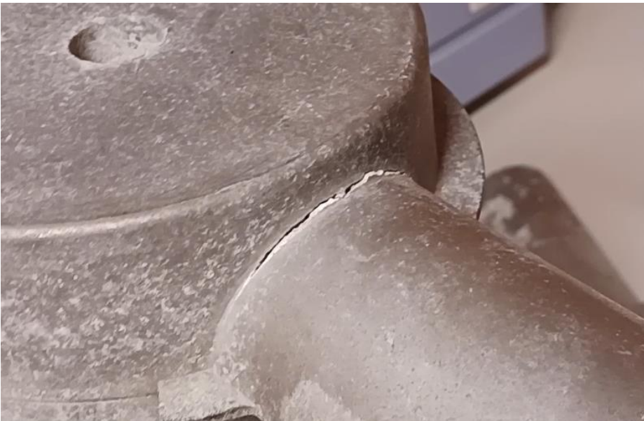
Figure 10 - Left Loading Failure
