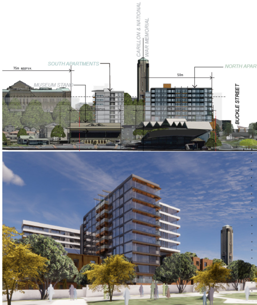
Figure 2.2: Alternating building alignment reduces the effects of mass from the north and east
