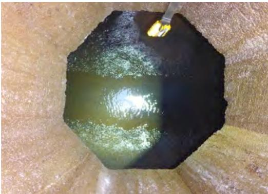
Measuring the atmosphere using a gas detector
