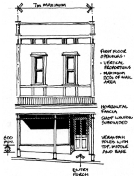
Compositional Principles of a Typical Existing Shopfront
