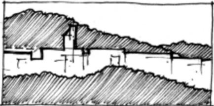
**G4** In the nominated zone at the centre of Area 1, a tower with floor areas generally not exceeding 800m<sup>2</sup> at any level above RL 130m may rise above the standard building envelope to an approximate height of RL 160m, subject to its siting, sculptural qualities and plan configuration being such that it makes a positive contribution to the overall form of the campus and ensures reasonable maintenance of views across the campus.
