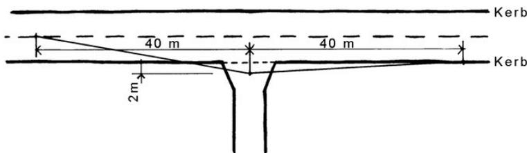
Within the area represented by the visibility splay, full visibility is required above a level of one metre above the level of the adjacent carriageway.
