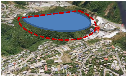
FIGURE 9 AREA (IN BLUE) POTENTIALLY SHELTERED TO 50% OF INCIDENT WIND SPEED DUE TO THE HEIGHT OF THE HILL TO BE REMOVED ABOVE THE HEIGHT OF HOMEBUSH ROAD OR MANDALAY TCE
