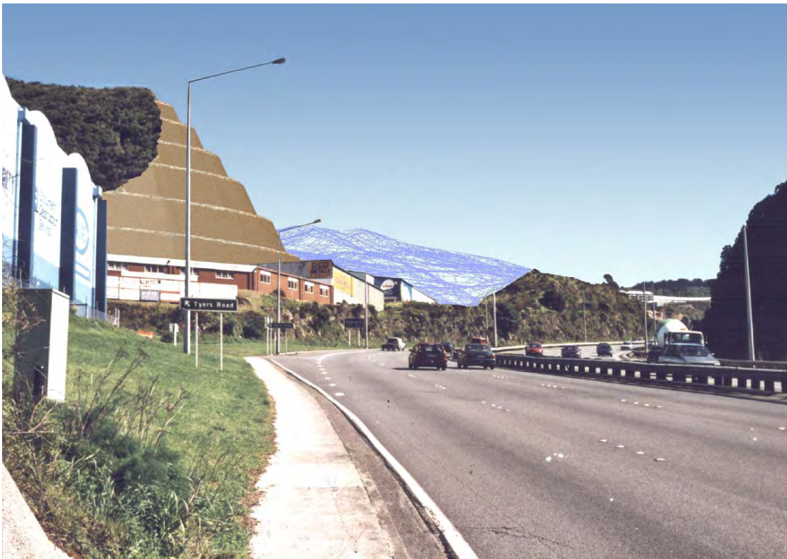
Simulation - View D : View north from northbound lane at the end of Stage 4. The simulated quarry face is based on the staging models in Figures 2(a) and (b). The final face will be finished with varied benching, gradients and ground conditions to appear more natural and aid plant establishment, as illustrated in Figure 11. The revealed landform of Broadmeadows is indicative, modelled from LINZ 20m topographical contour data.
