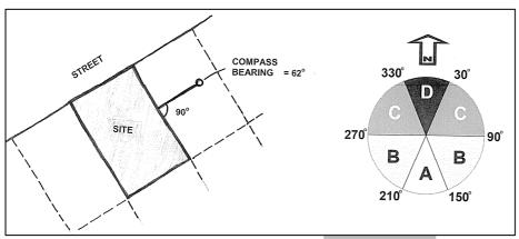
The orientation of a boundary is determined by the compass true north bearing of a perpendicular line drawn outwards from the boundary. In the example above the compass bearing is 62° so the building recession plane angle for Sector C would apply along this boundary.
