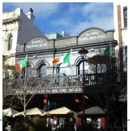
This building was strengthened in 1993 but the issue of pounding was not addressed. Current standards rate this at 37% of the current code, but a significant increase can be made by addressing the pounding hazard.
