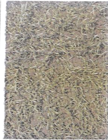
Grass master fibres, with all the natural grass removed.
