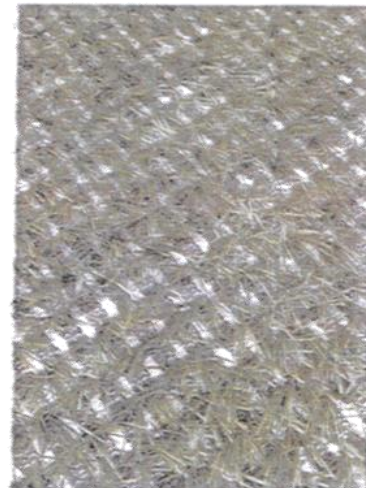
Hybrid, open weave carpet into which grass is established and sand incorporated.
