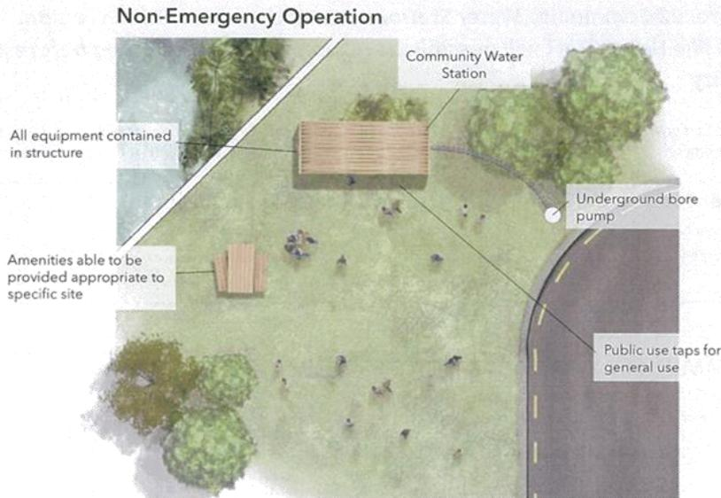
Under normal operation, emergency equipment is stored within a structure that is hidden inside a wooden shell to minimise impact on the area's natural character. The modular design allows for additional amenities to be installed, such as public taps, seating areas, and other features.
