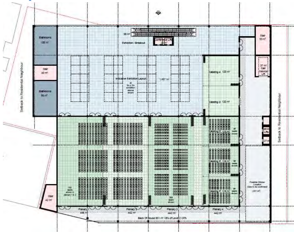
Figure 10: Floor plan of proposed convention centre in the combined movie museum development
