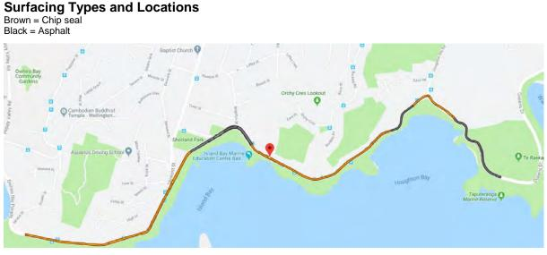
As can be seen from the above map we have used asphalt on the higher stress areas and chip seal on the remainder. This is in line with our asset management practices.
