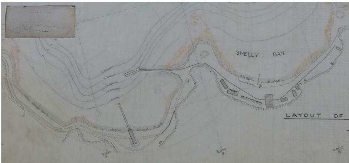
**Fig. 6** Extract map view showing the layout of the Shelly Bay buildings ca 1900s (full image inset). The tramway extends from the wharf jetty around to the north bay. Note the torpedo boat-shed and slipway in the south bay built in 1898.
