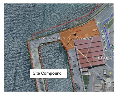
The compound would be erected in an area north of the main wharf where 3x welfare containers will be sited plus 1 x tool shed, these will be double stacked to save space. These facilities will be powered by a diesel generator and the ablution block will have a septic tank; it is possible that these services may be provided by mains connection. The compound will be fenced with 2m high site fencing and hoarded with scrim cloth. The foundations for this may be excavated into the ground.
