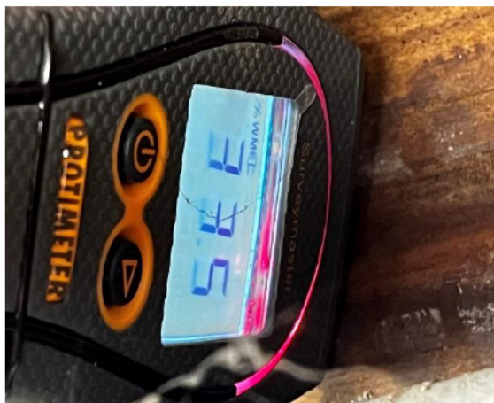
2.17 Elevated moisture readings
