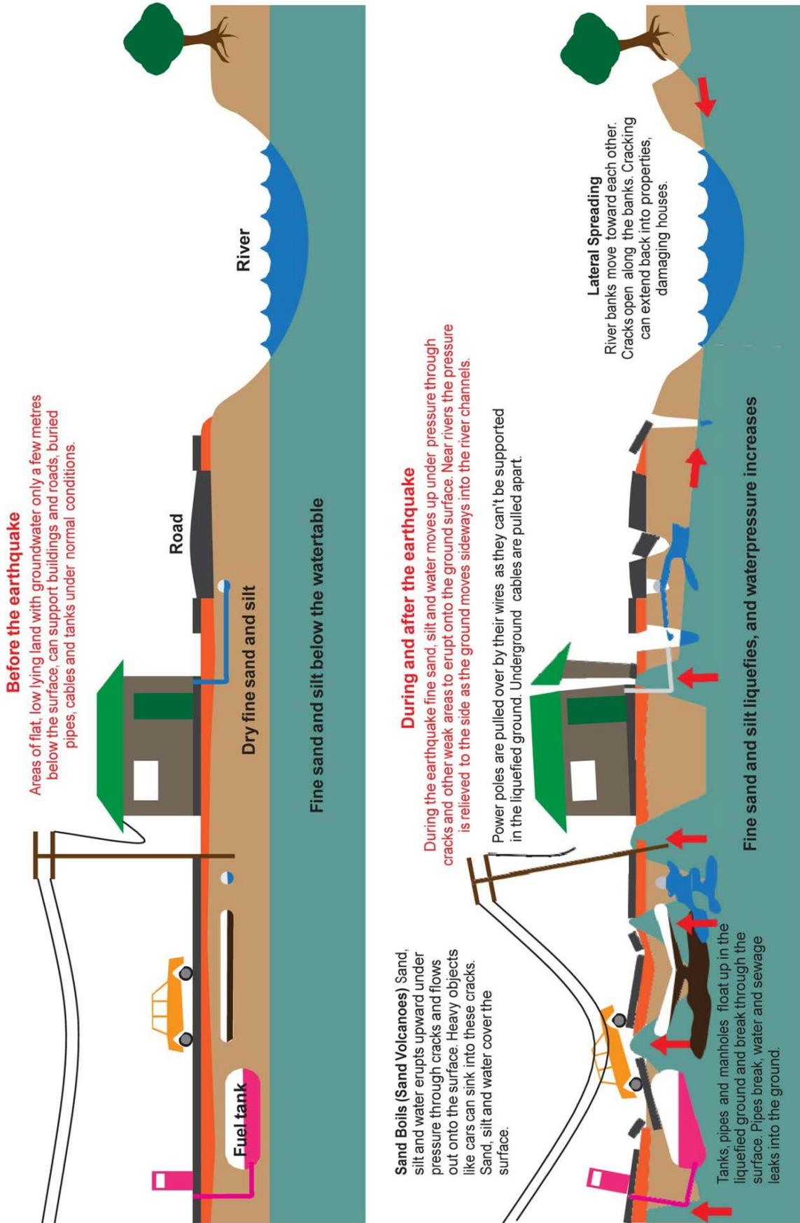
Figure 2.1 Diagrammatic illustration of liquefaction and its effects (IPENZ [date unknown]).
