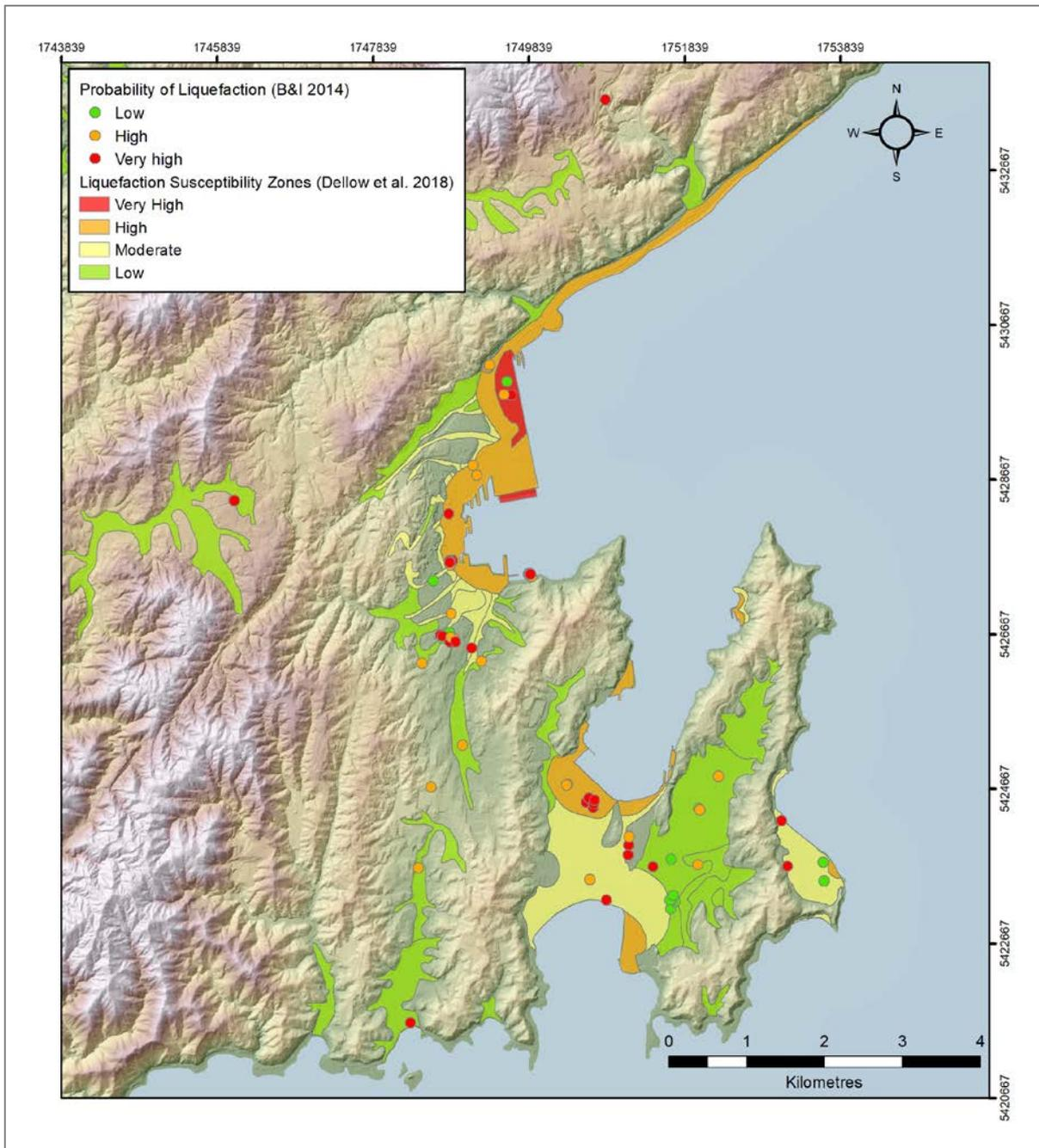
Figure 7.3 Overall probability of liquefaction occurring in selected CPTs in the Wellington City Council jurisdiction, based on a 10% in 50 years probabilistic seismic hazard for PGA with the associated average magnitude (7.3). The probability is calculated using the Boulanger and Idriss (2014) liquefaction-triggering assessment method. It is important to note that the absence of liquefaction does not imply that the area is safe from deformation.
