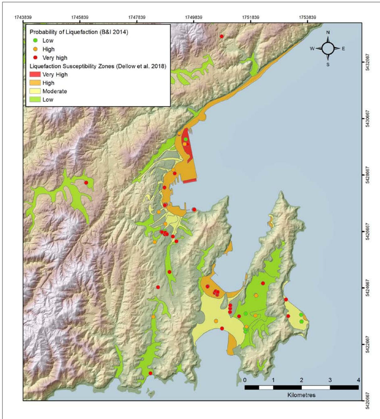
Figure 7.2 Overall probability of liquefaction occurring in selected CPTs in the Wellington City Council jurisdiction, based on an 84<sup>th</sup>-percentile mean peak ground acceleration scenario hazard for the 2010 NSHM Hikurangi-Wellington minimum source (magnitude 8.1). The probability is calculated using the Boulanger and Idriss (2014) liquefaction-triggering assessment method. It is important to note that the absence of liquefaction does not imply that the area is safe from deformation.
