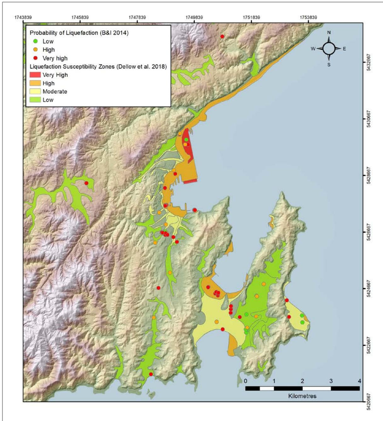
Figure 7.1 Overall probability of liquefaction occurring in selected CPTs in the Wellington City Council jurisdiction, based on an 84<sup>th</sup>-percentile mean peak ground acceleration scenario hazard for the 2010 NSHM Wellington-Hutt Valley fault source (magnitude 7.5). The probability is calculated using the Boulanger and Idriss (2014) liquefaction-triggering assessment method. It is important to note that the absence of liquefaction does not imply that the area is safe from deformation.
