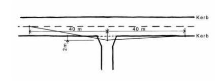
Within the area represented by the visibility splay, full visibility is required above a level of one metre above the level of the adjacent carriageway.
