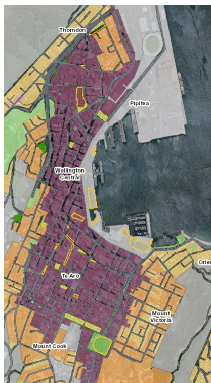
Figure 11: Minimum sunlight access requirements control applying to the WFZ and CCZ public spaces as shown in yellow hatching.
