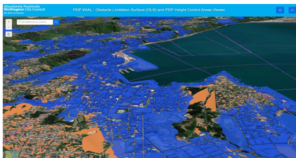
Figure 1 – An Indicative 3D Visual Representation of Parcels (and Building Envelopes) Where Plan Enabled Building Heights (Notified PDP) Exceeds Proposed WIAL Height Restrictions (8m + 30m) for WIAL1
