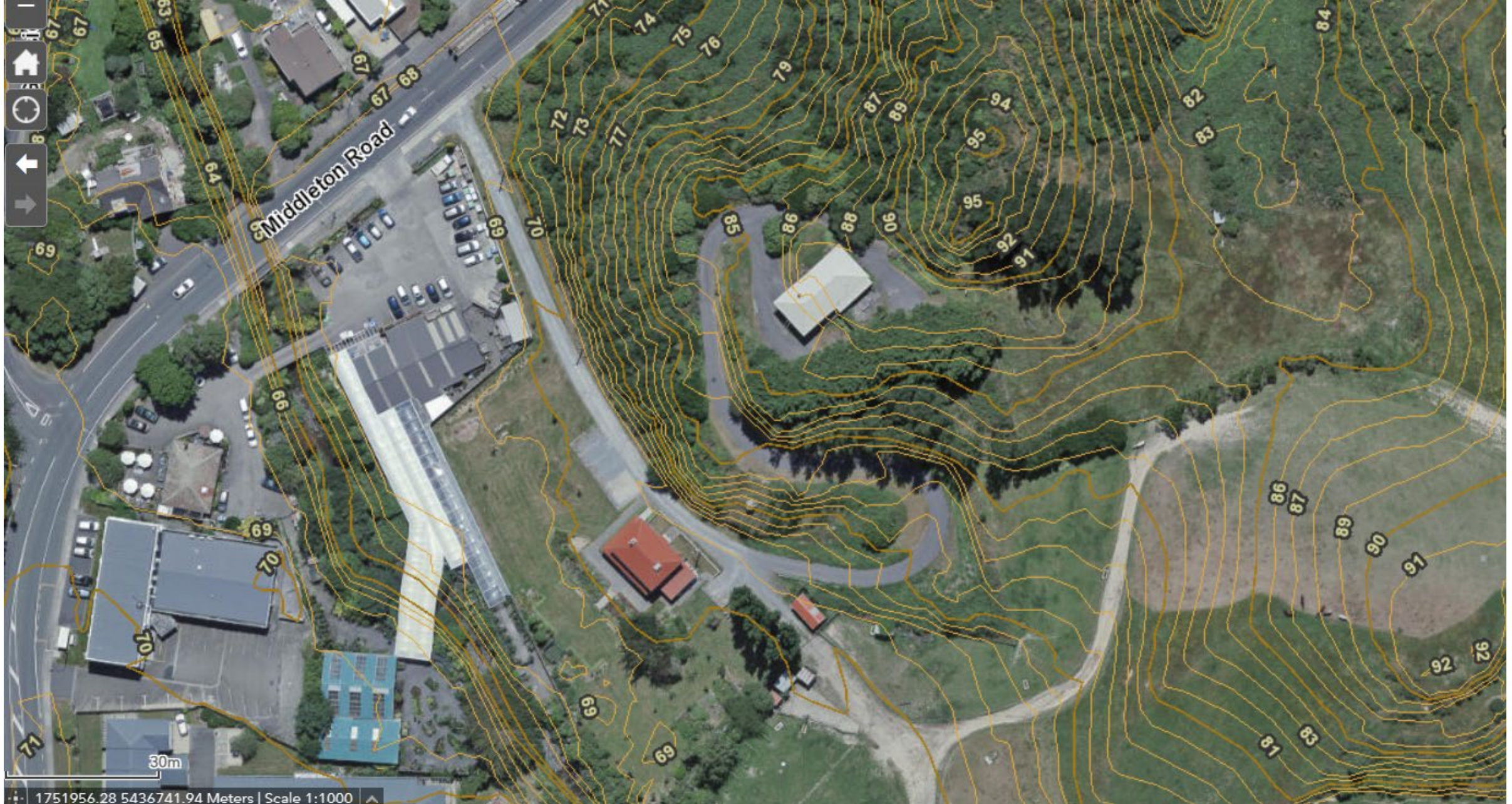
Contours - Wellington City Council online map 10-20 m heights on north side of reserve – natural recession plane at entrance
