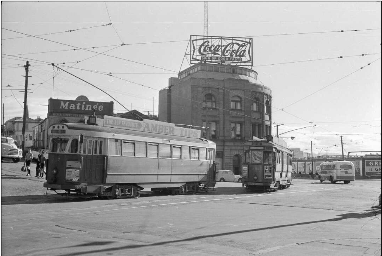
“Wellington trams passing Lambton Quay”: a view of some of the last operational trams in 1963. Note the crisscross of overhead wires and the trolley pole connected from the car to the wires (A. E. Smith, 1963).
