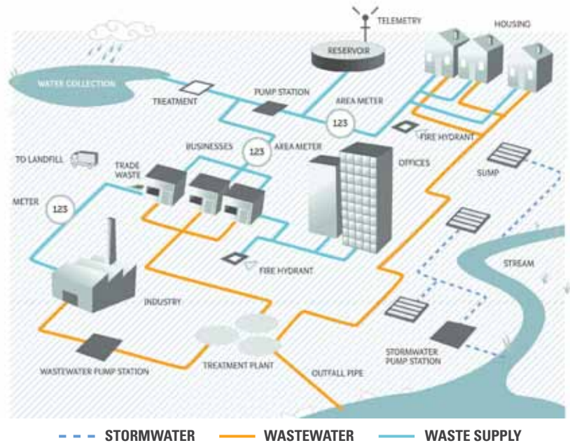
ELEMENTS OF THE 'THREE WATERS' NETWORK
