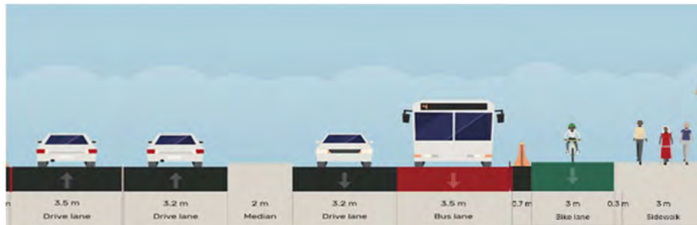
Option 1 - Hutt Road Indicative Cross Section
