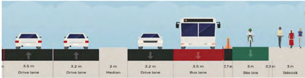
Figure 5-15 Option 4 – Thorndon Quay Indicative Plan and Cross Section
