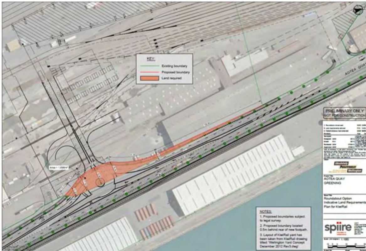
Figure 16: Proposed Layout for Turnaround facility at Aotea Quay
