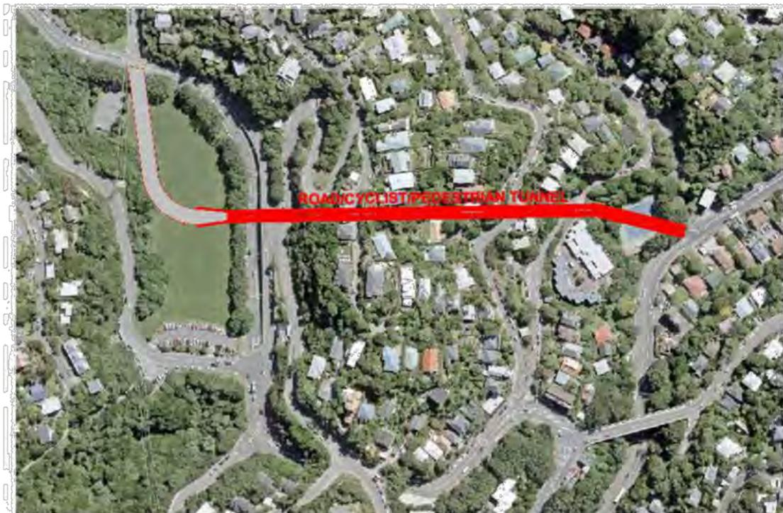
The length of the tunnel as shown is approximately 350 metres, and the length of the curved ramp to the Curtis Street intersection is approximately 150 metres.
