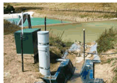
Above: Auto sampling equipment collects water samples from the inlet of the pond, it's then analysed for sediment content.
