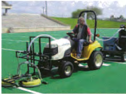
Deep vacuuming to remove worn fibre and foreign bodies.
