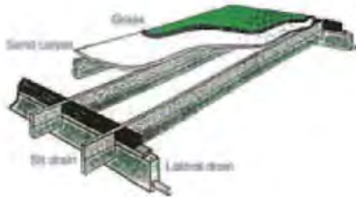
Sand Carpet Profile: Sand carpets are designed specifically to drain freely.
