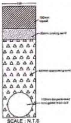
Lateral Drains: Move water to collector drains
