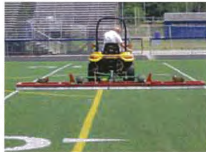
Grooming which replaces dislodged crum-rubber for even surface.
