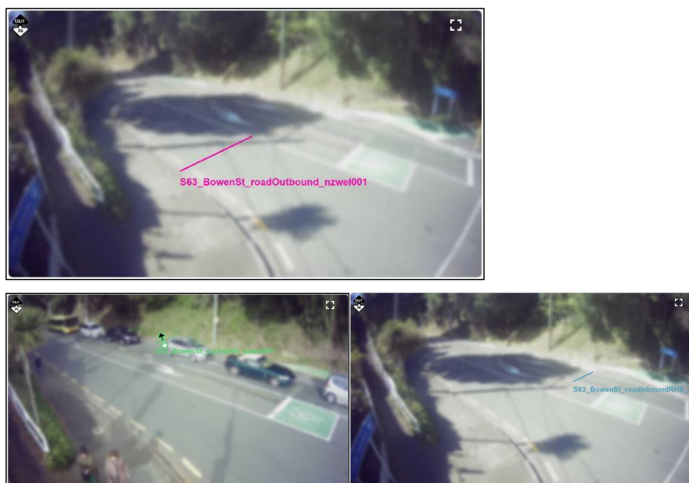
Figure 5. VivaCity sensor views in Bowen Street covering citybound (upper image) and Karori bound (lower image)
