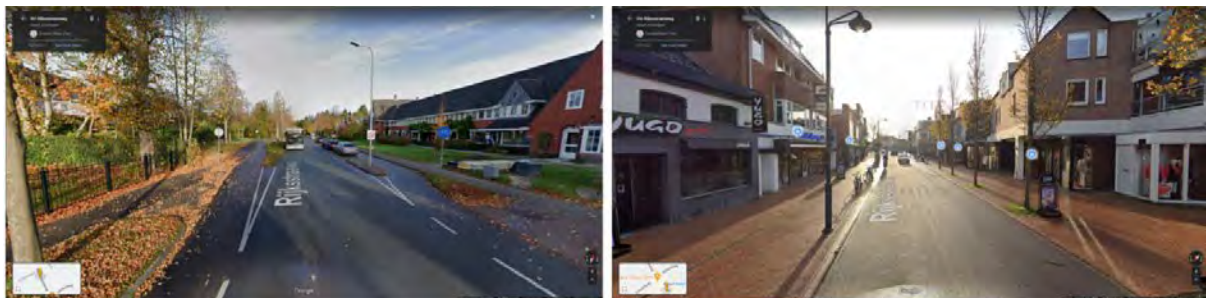
[Rijksstraatweg Groningen at Haren] Separated bike line (left image) merges onto a shared road (right) that used to have separate bike lanes, but cyclists and motorists weren’t getting enough practice interacting so the lanes were removed.
