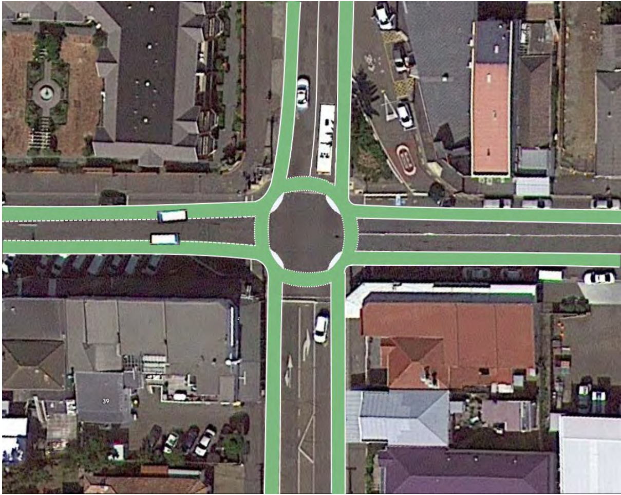
Dutch junction design on Onepu / Coutts Street. Note Coutts street towards the airport is shown with dashed lines as it may be too narrow for bike-only lanes if parking isn't removed.
