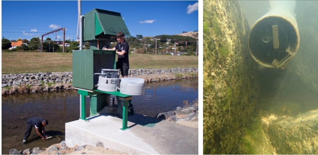
Porirua Stream at Town Centre flow monitoring site. Automatic water sampler in its housing and the turbidity sensor deployed in the stream (left) and (right) a close-up of the turbidity sensor deployed in the stream
