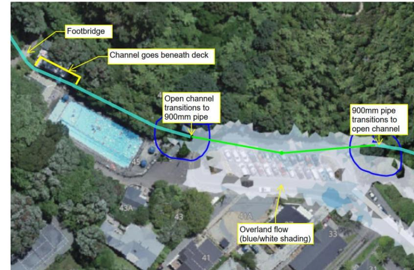
Figure 3.5 Wellington Water model results for the present-day 10% AEP rain event, provided by Wellington Water and marked up by T+T.
