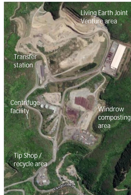
Figure 3-6 Southern Landfill – existing layout
