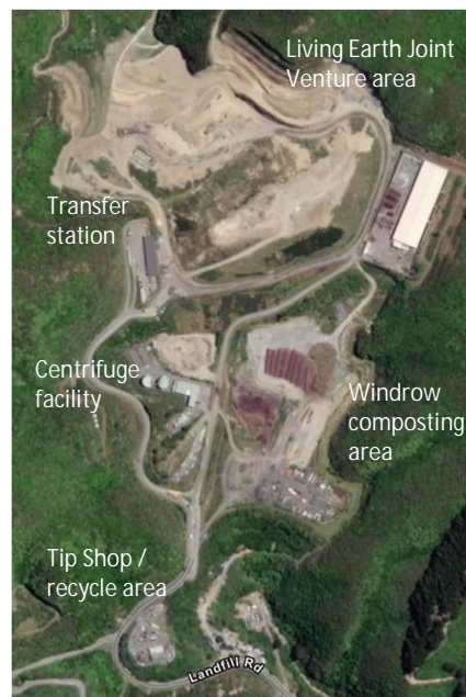
Figure 3-6 Southern Landfill – existing layout
