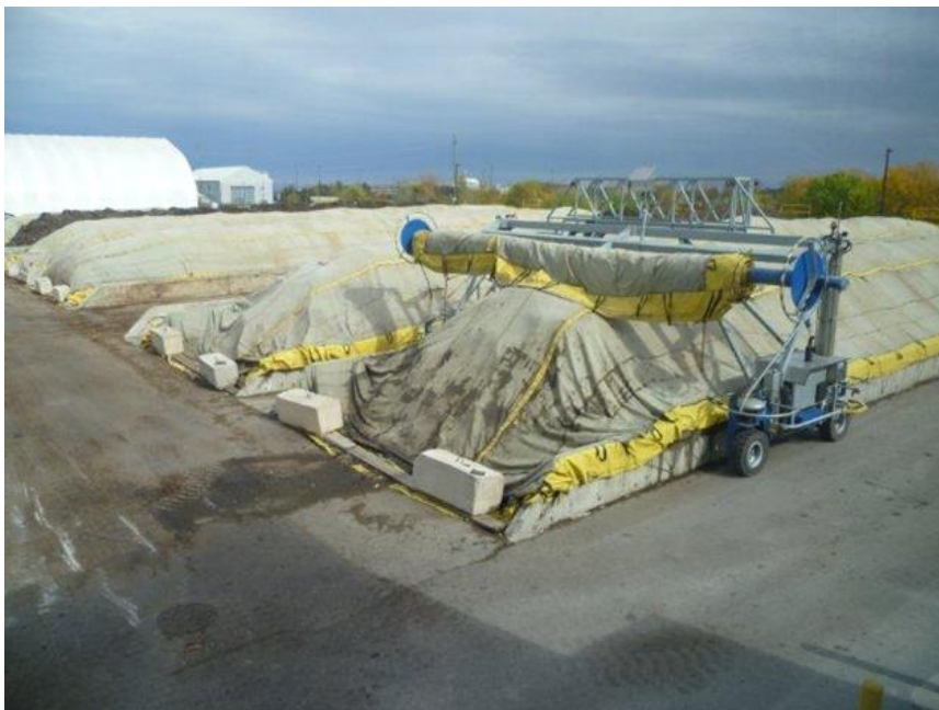
Figure 5 – example of covered aerated pile
