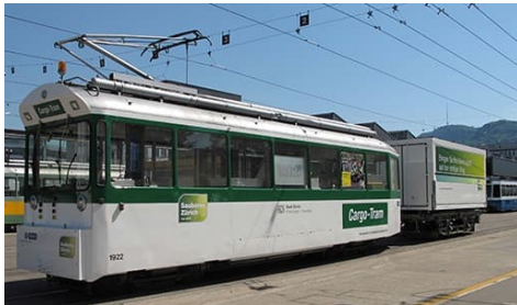
Figure 3-10 Cargo-tram recycling collection
