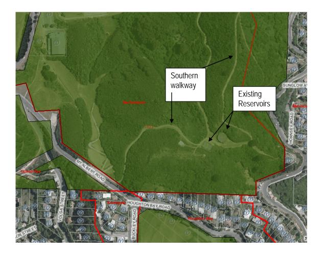
**APPENDIX 2 - Proposed Easement Area**The easement area shown orange and yellow encompasses the two tanks and immediate pipe work over a total area of 1771m2. The blue and yellow areas are an existing telecom occupation.
